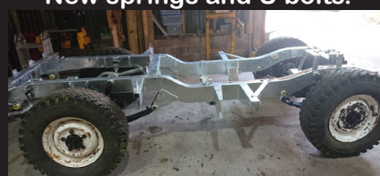
New chassis from Richard's, axles mounted.
