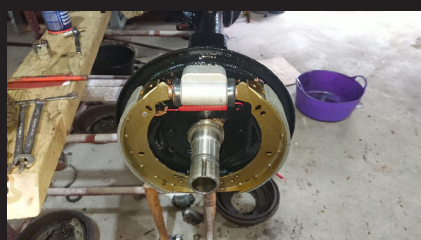
All new brake cylinders and shoes.
