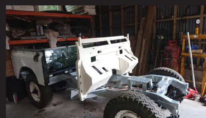
Engine stripped, painted and rebuilt. Painted body starts to come together
