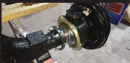
Axle rebuild , replaced swivel housing, seals and bearings.
